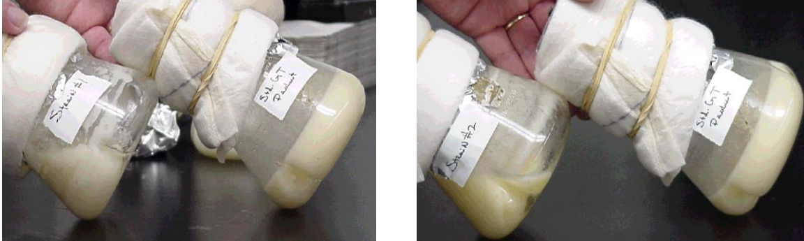
Figures 3 & 4 - Fat Degradation capabilities of two EBtech isolates compared to a commercially available grease trap product
